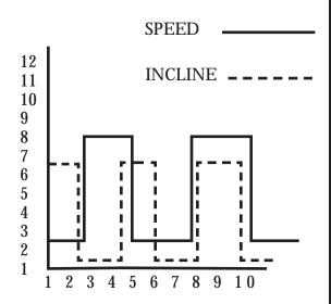
The **Cross Training Program** is designed to control the walking belt speed and elevation inversely in alternating segments.
